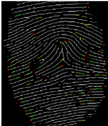
Figure 20 Real Minutiae after false removal
